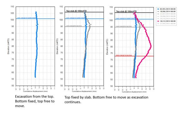
The graph above shows ShapeArray measurements from a retaining wall where construction started with displacements referenced to the bottom of the instrument and then changed to the top of the instrument when the top slab was added.
