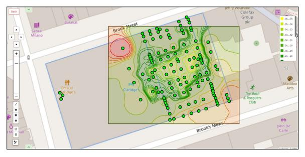
All of the measurements are collected remotely and can be presented on our web-based Geodaisy® software (shown above) with contours to make it easy to understand where the movements are happening.
