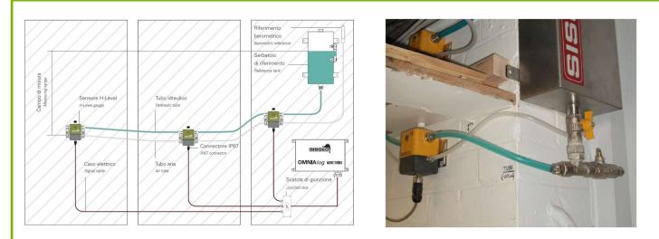
The pictures show how liquid levelling sensors are connected to a fluid reservoir and detect relative movements between the sensors. One sensor and the reservoir are located in a stable location or where the movements can be independently checked and used as a reference point. The sensors are very sensitive and cannot tolerate large changes of absolute elevation so when this occurs two sensors are positioned alongside each other and the displacements are transferred virtually.
